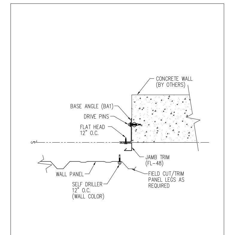
NOTE: USE POWER DRIVEN FASTENERS SUCH AS RAMSET (OR EQUAL).  $0.140 \, \text{Ø}$  STRAIGHT SHANK W 1 1/4" PENETRATION AND MIN. ALLOWABLE SHEAR OF 220# (2'-0" O.C.)(NOT BY GWB)
