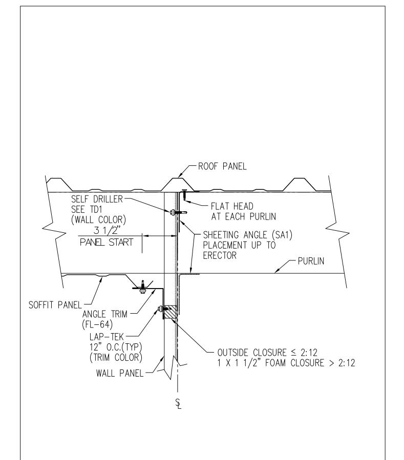
NOTE: FIELD NOTCH WALL PANEL AROUND PURLINS AND EAVE STRUTS NOTE: FIELD SLOPE CUT WALL PANELS AS REQUIRED FOR ROOF SLOPE
