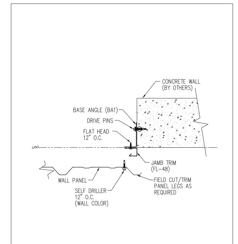
NOTE: USE POWER DRIVEN FASTENERS SUCH AS RAMSET (OR EQUAL). 0.140¢ STRAIGHT SHANK W 1 1/4" PENETRATION AND MIN. ALLOWABLE SHEAR OF 220# (2'-0" O.C.)(NOT BY GWB)
