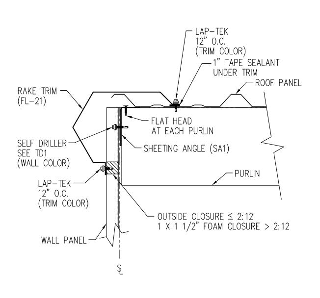
NOTE: FIELD SLOPE CUT WALL PANELS AS REQUIRED FOR ROOF SLOPE
