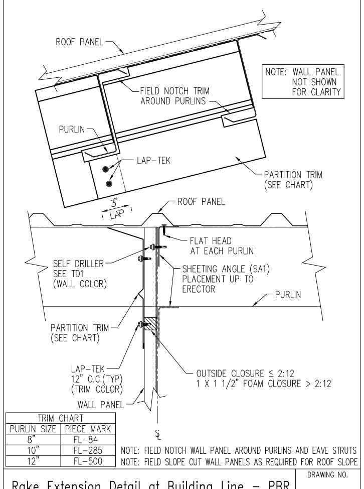
Rake Extension Detail at Building Line — PBR
