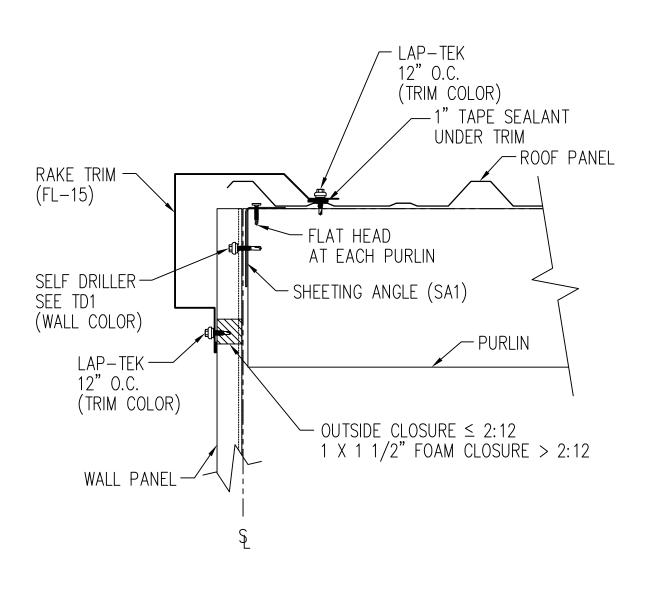
NOTE: FIELD SLOPE CUT WALL PANELS AS REQUIRED FOR ROOF SLOPE
