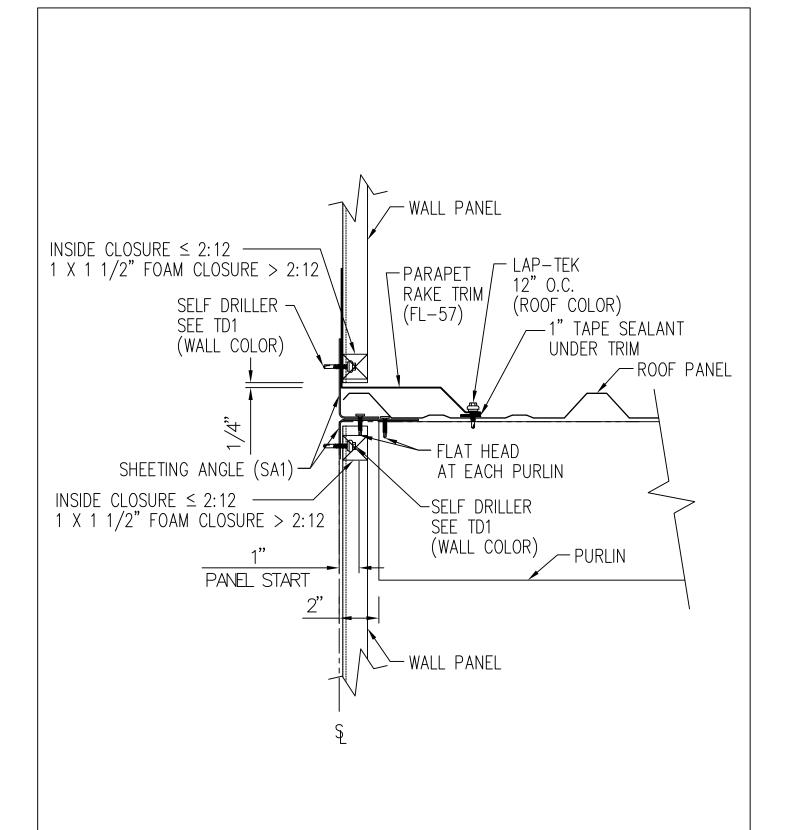
NOTE: FIELD NOTCH WALL PANEL AROUND PURLINS AND EAVE STRUTS NOTE: FIELD SLOPE CUT WALL PANELS AS REQUIRED FOR ROOF SLOPE
