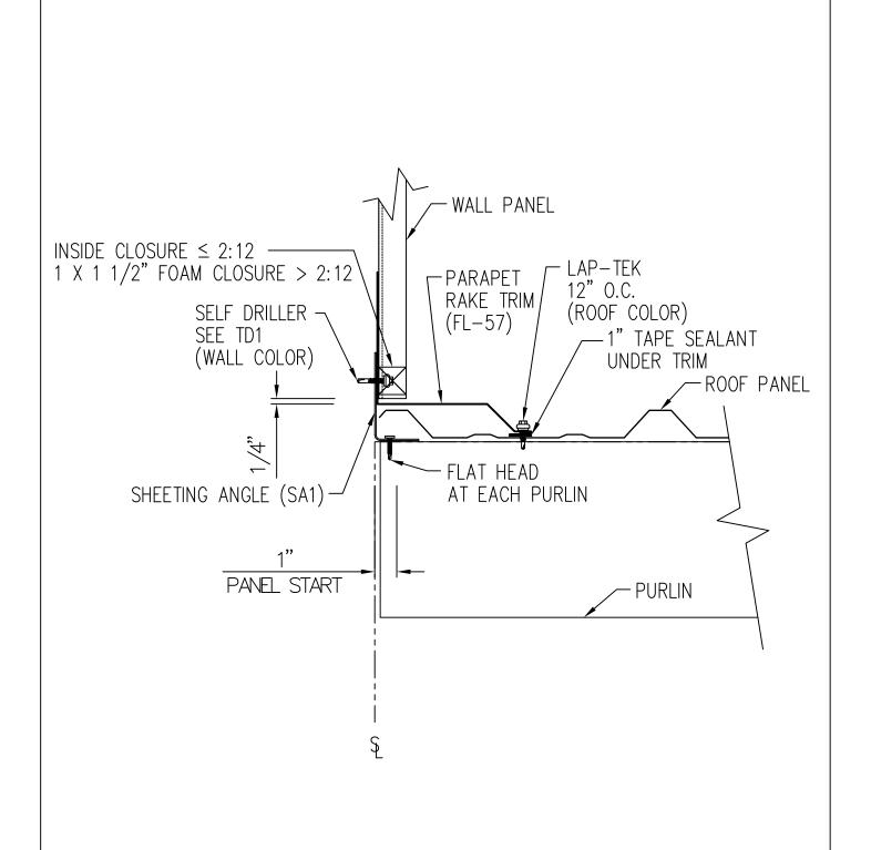
NOTE: FIELD SLOPE CUT WALL PANELS AS REQUIRED FOR ROOF SLOPE
