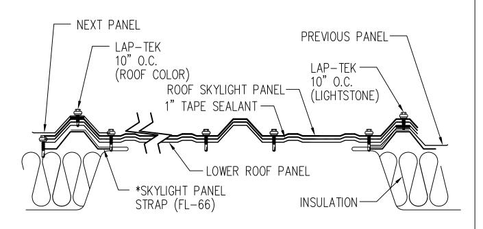
NOTE: ALL ROOF SKYLIGHT PANELS ARE FIELD LOCATED.
