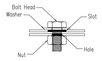
Slot to Hole Connections
