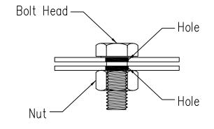
Hole to Hole Connections
