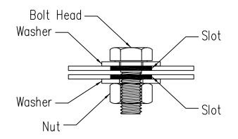
Slot to Slot Connections
