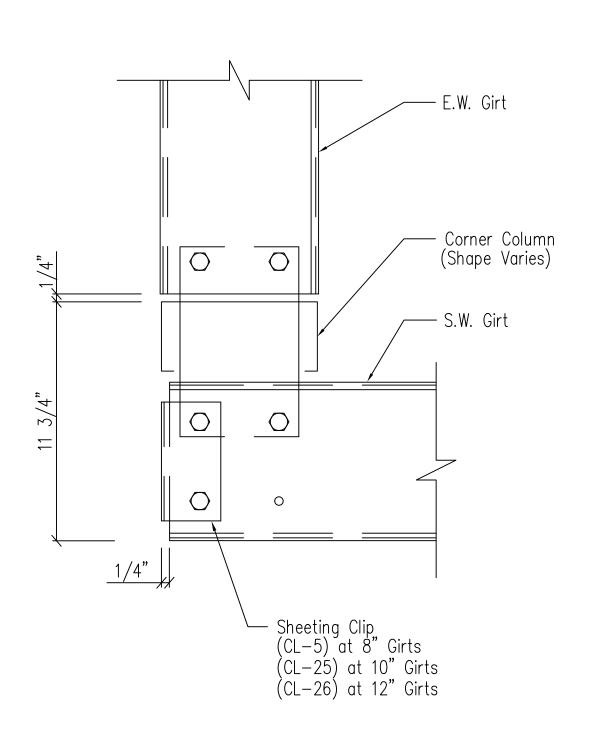
Note: All connection bolts are 1/2" x 1 1/4" machine bolts unless noted.
