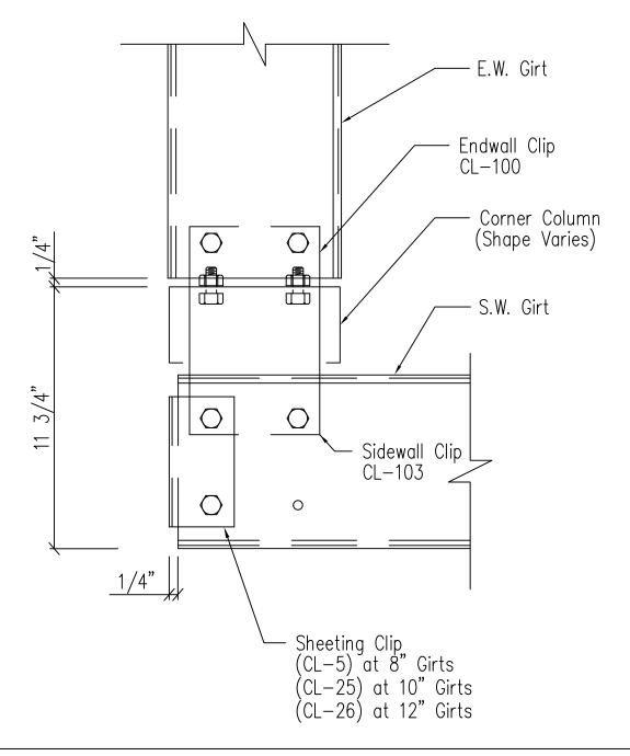
ERECTOR NOTE: IF CLIP BOXES ON BUILDING ELEVATION VIEW(S) ARE BELOW THE INTENDED GIRT LINE, THE CLIP(S) IN REFERENCE ARE TOED DOWN. IF ABOVE THE GIRT LINE, THEN TOED UP.
