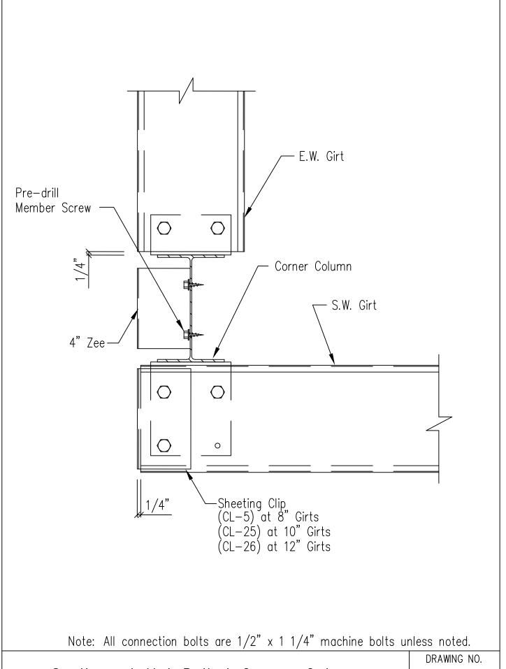
Section at Hot Rolled Corner Column
