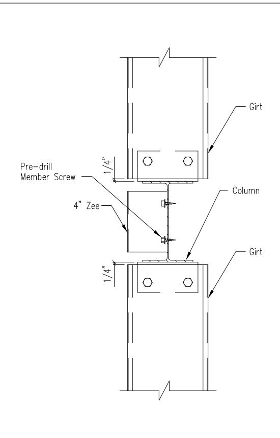
Note: All connection bolts are 1/2" x 1 1/4" machine bolts unless noted.
