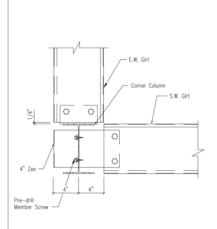
Note: All connection bolts are 1/2" x 1 1/4" machine bolts unless noted.
