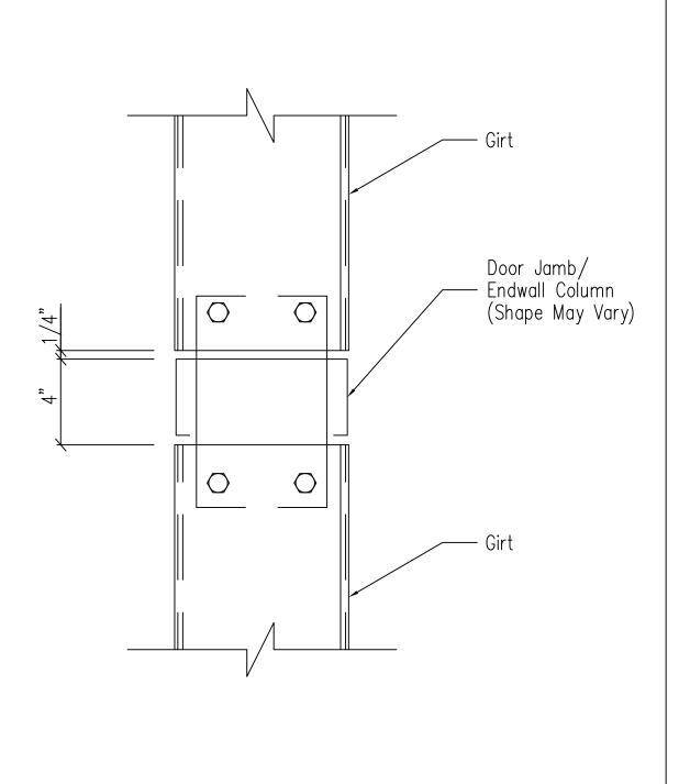
Note: All connection bolts are 1/2" x 1 1/4" machine bolts unless noted.
