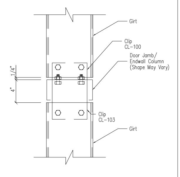
ERECTOR NOTE: IF CLIP BOXES ON BUILDING ELEVATION VIEW(S) ARE BELOW THE INTENDED GIRT LINE, THE CLIP(S) IN REFERENCE ARE TOED DOWN. IF ABOVE THE GIRT LINE, THEN TOED UP.
