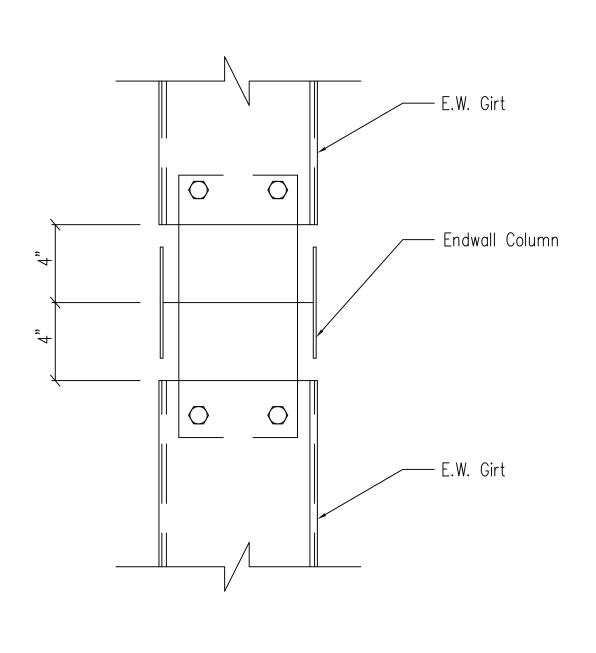
Note: All connection bolts are 1/2" x 1 1/4" machine bolts unless noted.
