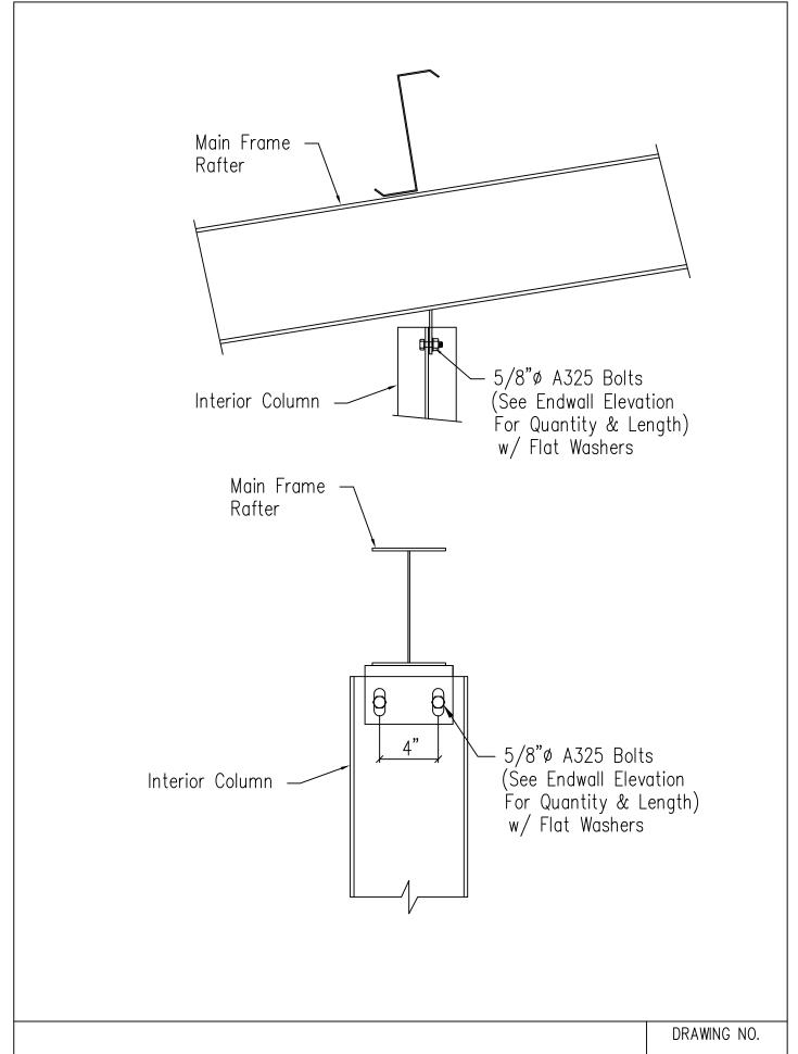
Hot Rolled Column to Main Frame Rafter
