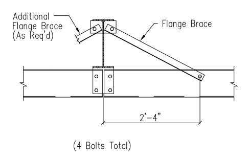
Note: All connection bolts are 1/2" x 1 1/4" machine bolts unless noted.
